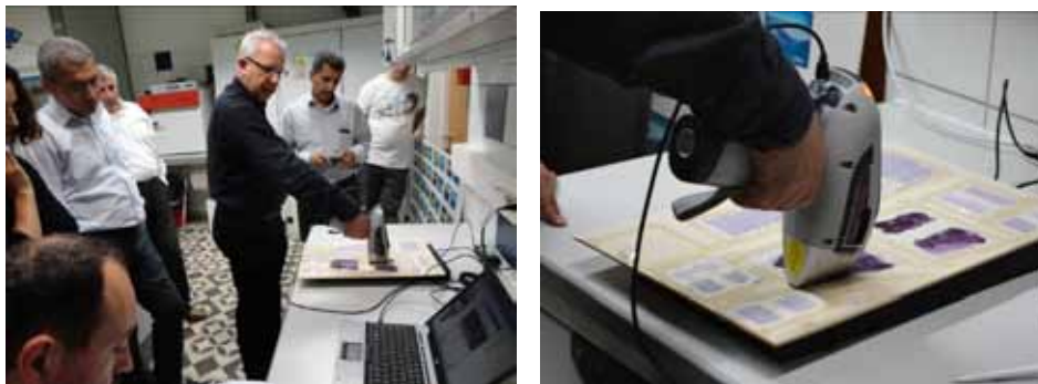
Photograph 3: Measurement of XRF spectra from pigments using a handheld spectrometer
