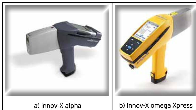
Figure 1: Used XRF handheld analyzers
